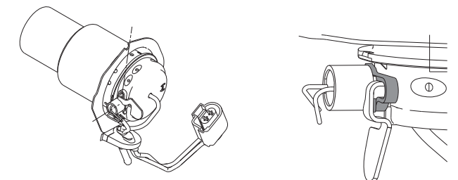
Fig. 913 Installing glow plug properly
